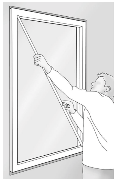
Fig 72. Check with spirit level.
