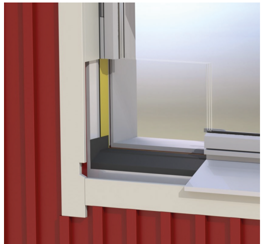
Fig 2. Cutaway of a window installed in a wall, showing the caulking, secondary seal, window sill etc.
