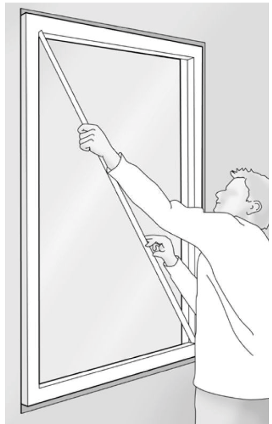
Fig 30. Diagonal measurements must be the same which guarantees good assembly
