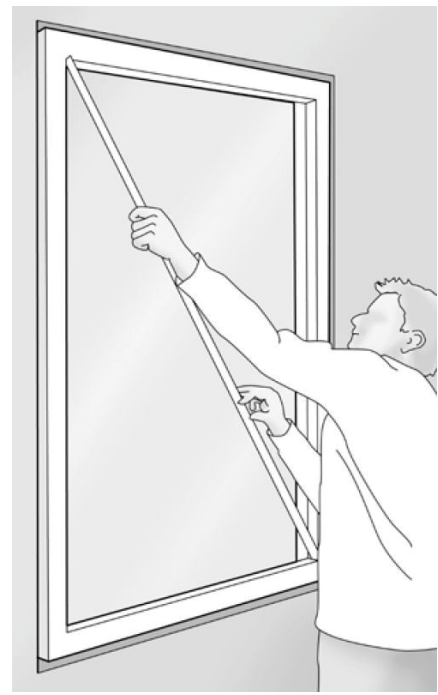
Fig 53. Diagonal measurement is important for the function of the door. The diagonal measurements must be equal.
