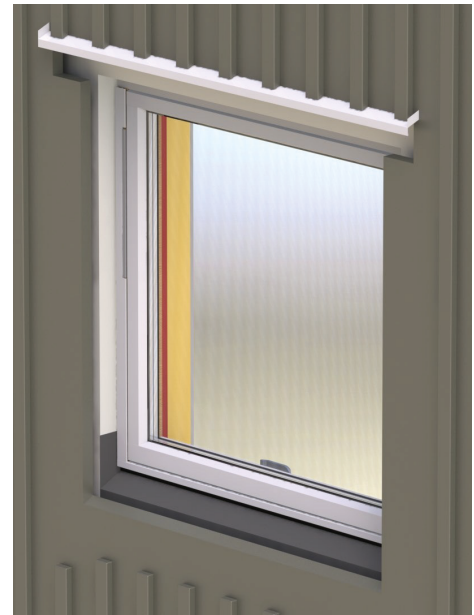
Fig 19. Secondary seal runs the full width of the window opening and 100 mm up at the sides. The seal prevents water from penetrating further into the construction.
