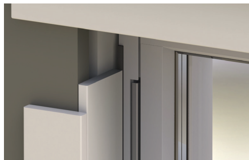
Fig 7. Flexible sealing tape between the window and the facade (external weather protection).
