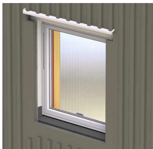
Fig 11. Secondary seal is drawn along the full width of the window opening and 100 mm up at the sides. The seal prevents water from penetrating further into the construction.
