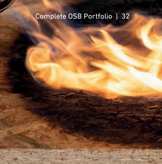
When exposed to flame, SWISS KRONO OSB/SF-B chars to form a fire-inhibiting layer.
